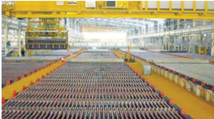
A copper electro-winning tankhouse that uses ISA PROCESS.
